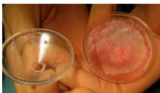
Filter Ø 48 mm - mesh opening 300 µm
